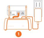
2. Install batteries and plug in power adapters to devices and sensors.
