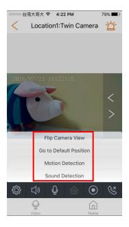
Flip Camera View: Flips the video feed to an inverted view.
