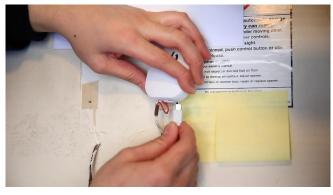
5.1.1.7 Mount the Garage Door Control Button via Double-sided tape or screws
