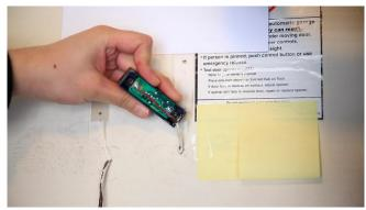
5.1.1.3 Unscrew wires from the opener (Note: The 2 wires will not cause a harmful electrical shock)
