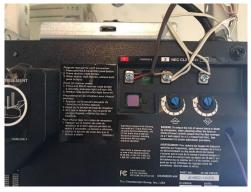
5.1.3.2 Loosen the garage door opener wire screws (Note: The 2 wires will not cause a harmful electrical shock)
