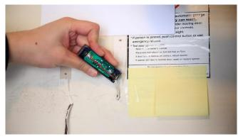
5.1.2.3 Loosen the screws (Note: The 2 wires will not cause a harmful electrical shock)
