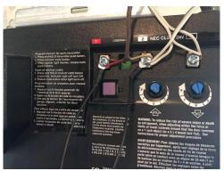
5.1.3.5 Insert wires into the Garage Door Control Button (one per hole, either hole choice is fine)
