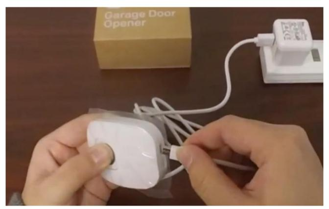
**3.1.2** While holding down the button, attach the power cable
