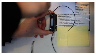
5.1.2.8 Insert wires into the Garage Door Control Button (one per hole, either hole choice is fine)
